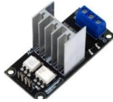
Gambar 7. Robotdyn AC Dimmer (Sumber : Mujahid Ahmad dkk., 2021 )
